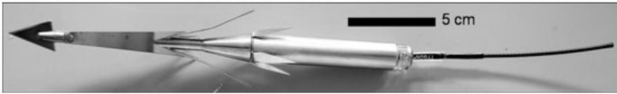
Figure 1. Satellite transmitter (Wildlife Computers implantable SPOT3/4) deployed in humpback whales in the Cook Island.
